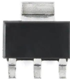
Figure 3.1.4. Real figure of AMS1117
