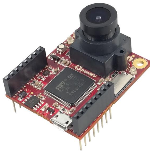
Figure 3.5.1. OpenMV4 H7 R2 Camera Module
