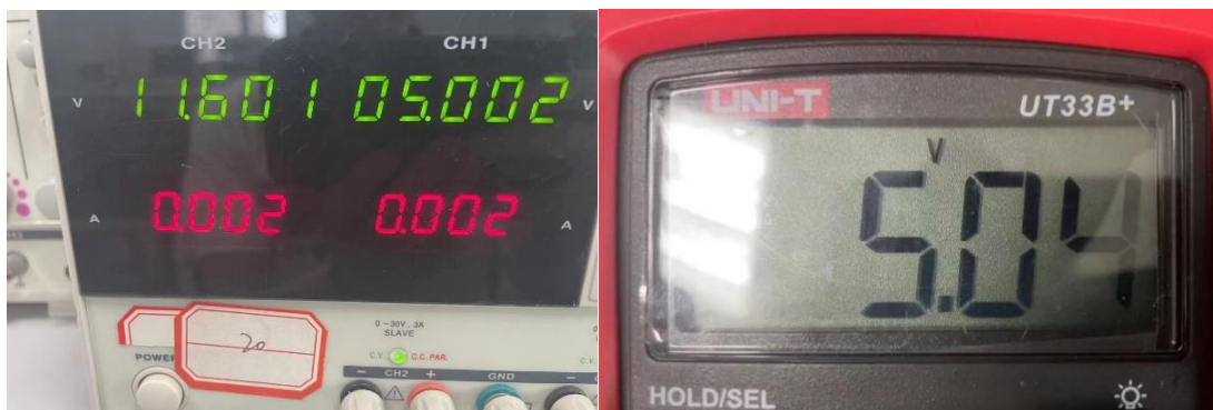
Figure 3.1.13. The 11.6V input (left) and output result of LM256 circuit(right)
