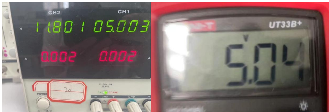
Figure 3.1.12. The 11.8V input (left) and output result of LM256 circuit(right)
