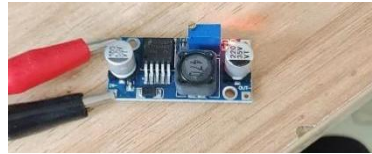
Figure 3.1.10. Real circuit for 12V to 5V transformer
