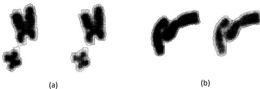
Figure 3.6.5. (a) Touching Chromosomes Separated by Opening Operation (b) Distinguish Chromosomes by Closing Operation
