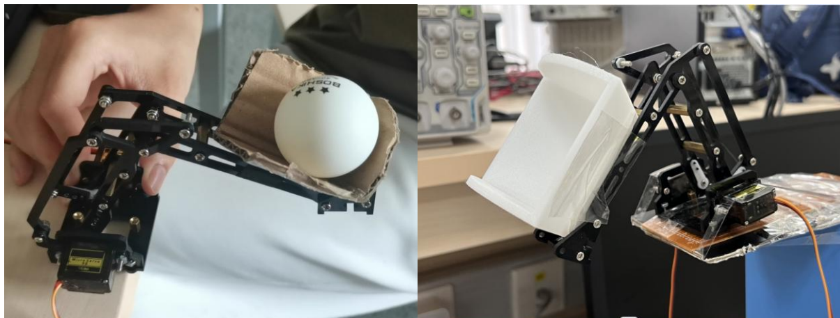
Figure 3.3.10. The improved design (left) and the final design (right)
