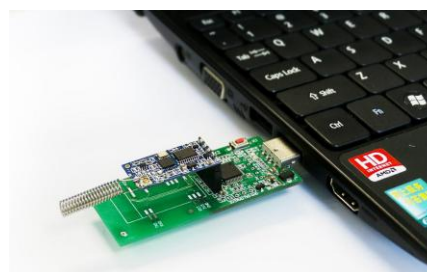
Figure 3.8. 2. Connection of MCU and HC-12(left) and connection of MCU and the computer(right)
