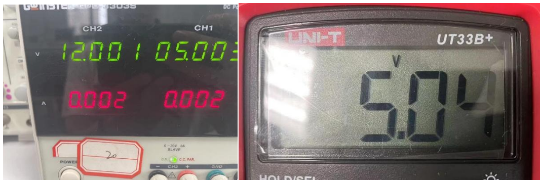
Figure 3.1.11. The 12V input (left) and output result (right) of LM256 circuit
