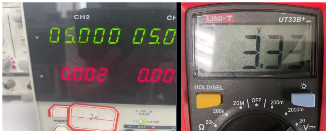
Figure 3.1.15. The input (left) and output result of AMS1117 circuit(right)
